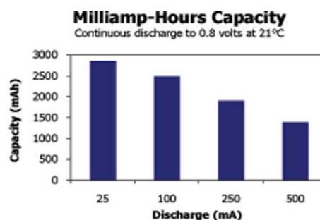
So, if you draw 25 milliamps from the battery, you get almost 3000 milliamp hours from your batteries. That means that you can last for 120 hours! (3000 milliamp-hours/25 milliamps = 120 hours) But how about if we draw 500 milliamps from the batteries? According to that graph, we only get a little over 1000 milliamp-hours. That means that the batteries will run for only a little over two hours. What a rip!
