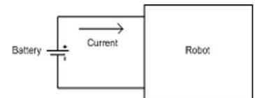
And the robot will keep drawing this current until your battery is dead. The amp-hour rating is basically the product (multiplication) of the current and the time it can provide that current:
